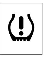
When a low tire pressure condition is detected, the TPMS illuminates the low tire pressure warning light on the instrument panel cluster.
